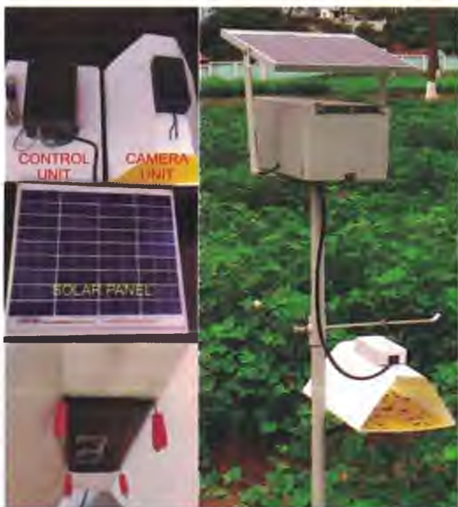
Multi Species pheromone septa and camera unit in the modified delta trap
