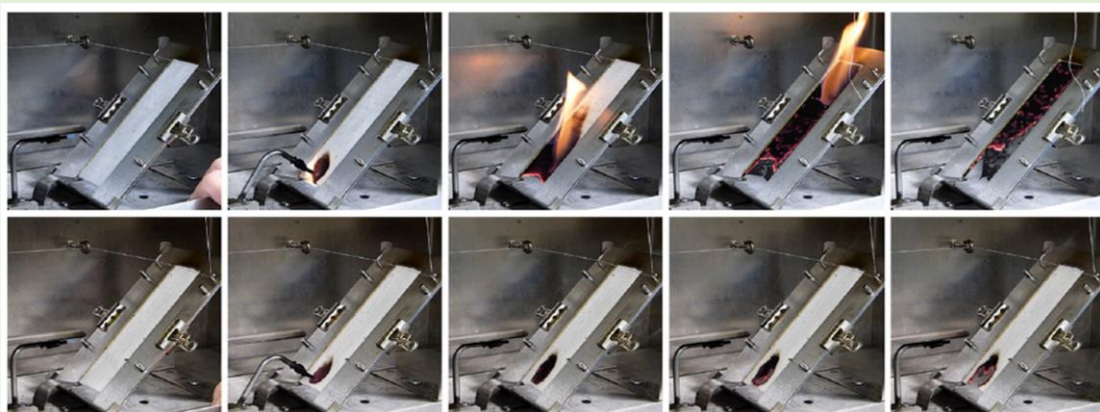
Fig.1 Time series of 45° incline flame test of non-woven fabrics from the MAGIC RILs with low & high HRC. Each image is 5 seconds apart. Top series is fabric made from RIL-225, which like all untreated textiles produced from conventional cultivated white cotton was fully consumed by flame in ~15 seconds. Bottom series is RIL-385, which self-extinguished.
