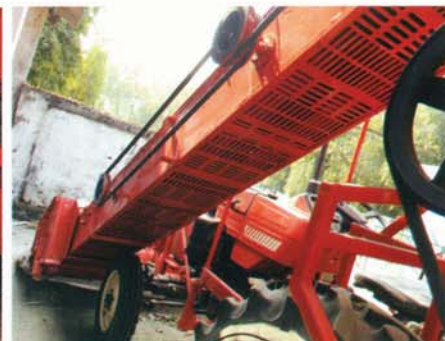
Slotted under cover for conveyor
